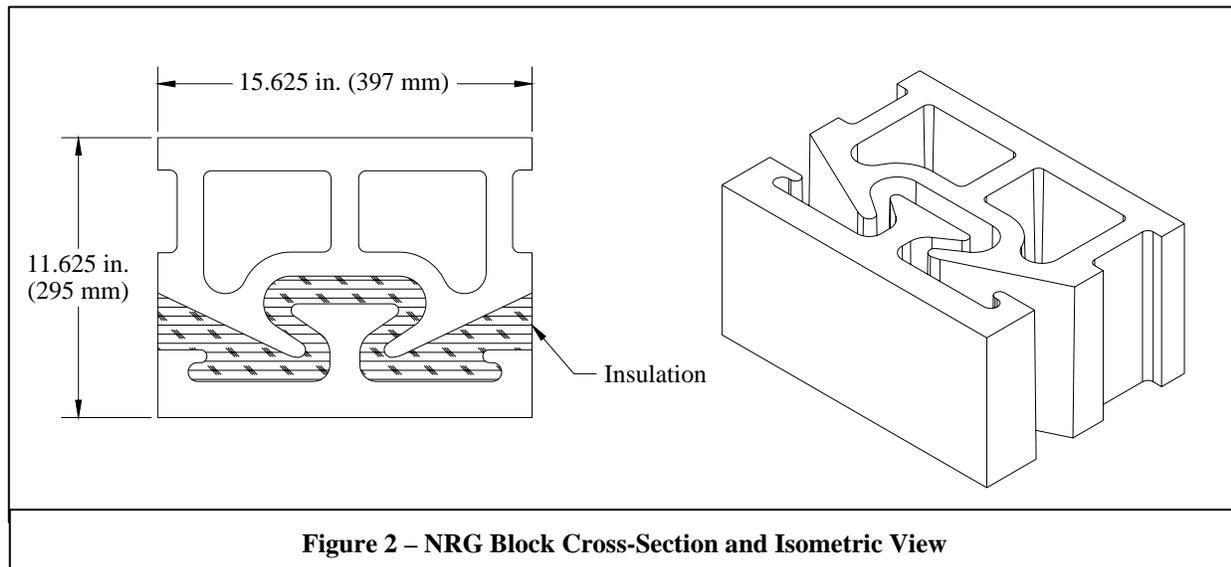
Based upon the dimensions of the full-size units as tested in this project, the net cross-sectional properties of the NRG units are summarized in Table 2. These values may be used for the purposes of designing and proportioning ungrouted masonry assemblies constructed with NRG block. Grouted section properties will vary based on spacing between grouted cells.
