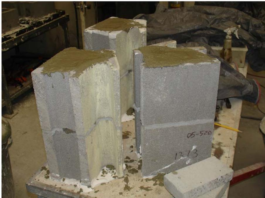
**Figure 3 – Reduced Size Solid Grouted NRG Prisms**
