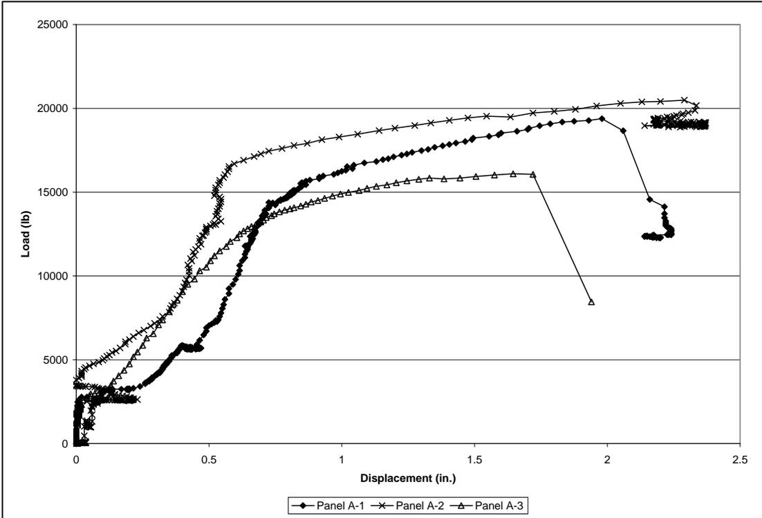
**Figure 7 – Load-Deflection Curves for Panel Set A**
