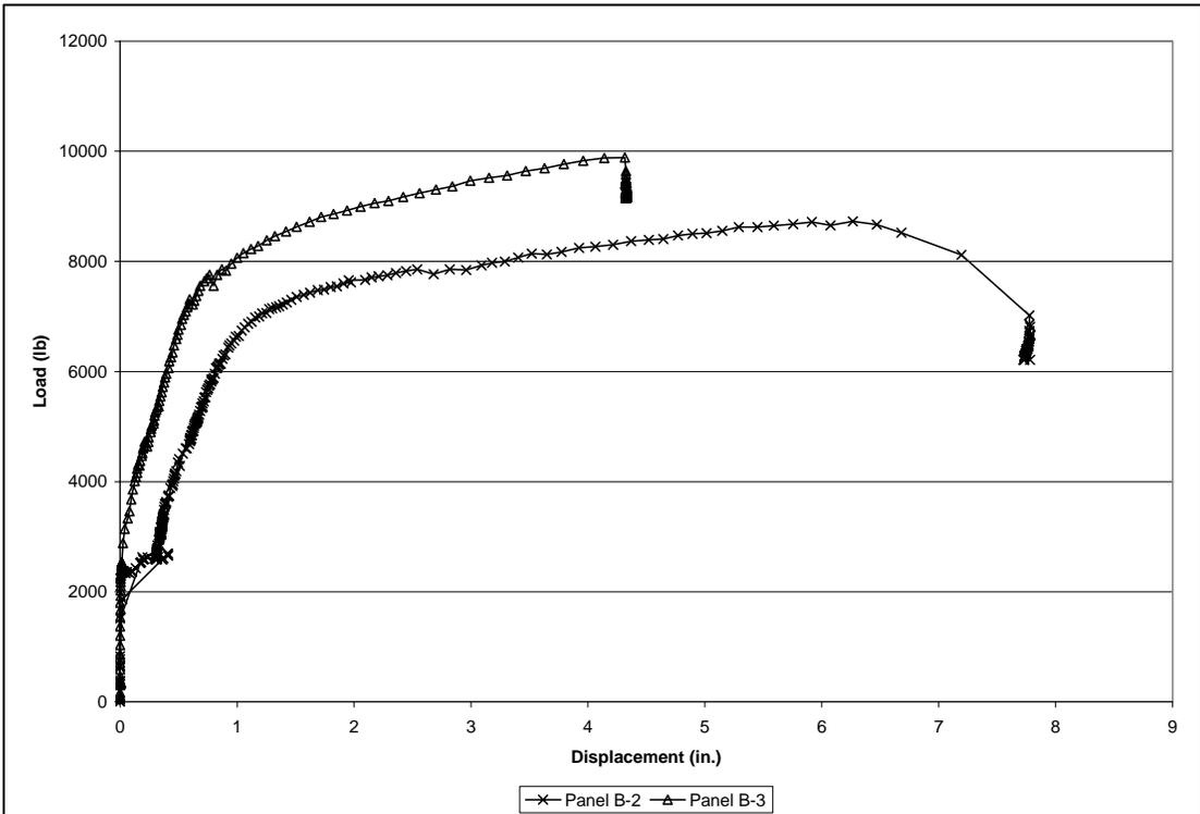
**Figure 8 – Load-Deflection Curves for Panel Set B**
